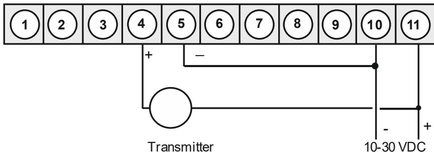
**M2 in combination with a 3-wire-sensor of 0/4-20 mA**
