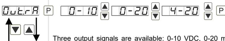
Three output signals are available: 0-10 VDC, 0-20 mA and 4-20 mA, with this function, the demanded signal is selected.
