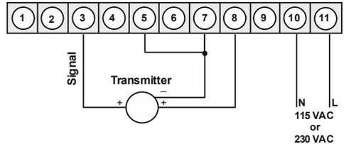
M2 with digital input in combination with 24 VDC sensor supply
