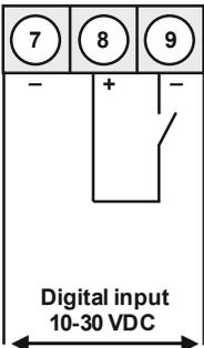
M2 with digital input and external voltage supply source
