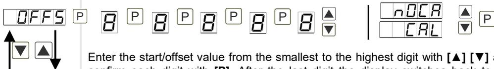
Enter the start/offset value from the smallest to the highest digit with [▲] [▼] and confirm each digit with [P]. After the last digit the display switches back to the menu level. If *SENS* was selected as input option, one can only select between *nOCA* and *CAL*. With *nOCA*, only the previously set display value is taken over, and with *CAL*, the device takes over both the display value and the analogue input value.
